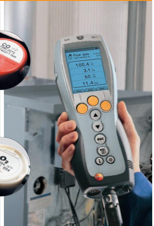
Fast monitoring of flue gas values in heating systems
