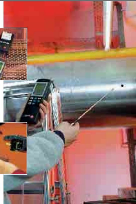
Fast and easy checking of SO 2 concentrations
