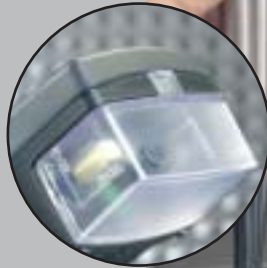
Condensate trap in instrument
