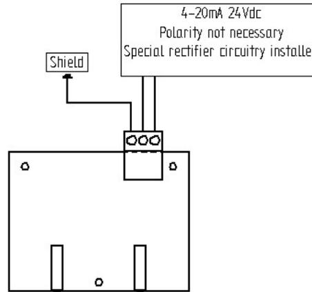
For calibration purposes, the signal may be monitored using either a local meter connected across TP1 and TP2 for mV or TP3 and TP4 for mA, or by a remote receiver. A small non-metallic screwdriver, with a 1.2 x 0.5mm tip, is required to adjust the potentiometers. Although in practise, the calibration procedure will be dictated by the hardware system employed, the following procedure will generally apply:-
